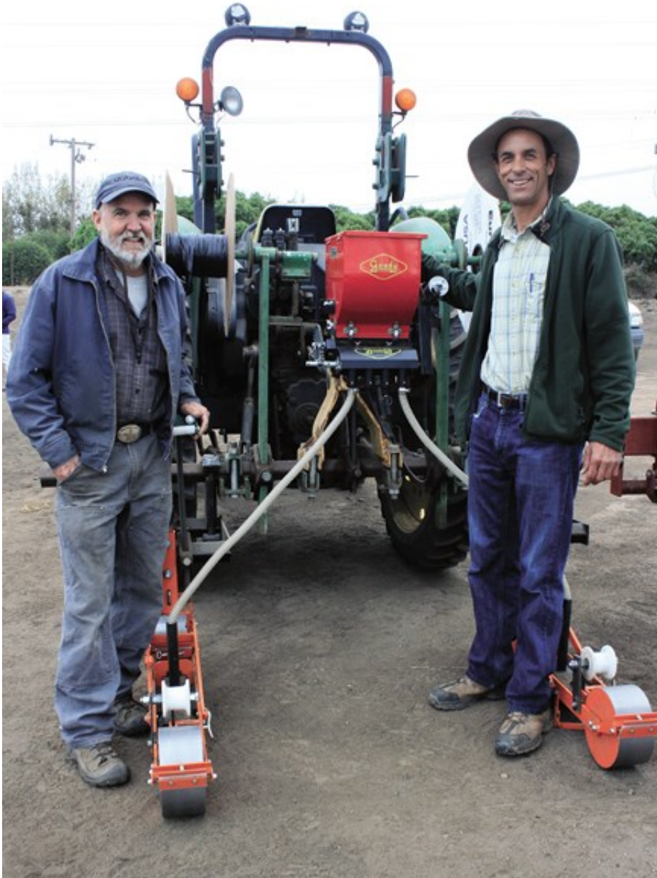
Eric Brennan, USDA research horticulturist, right, and Jim Leap, USDA agricultural science research technician, stand with their new Salinas planter-cultivator that can cultivate the furrow, plant a row of cover crop seeds and lay the drip line to germinate the seeds in a single pass.
